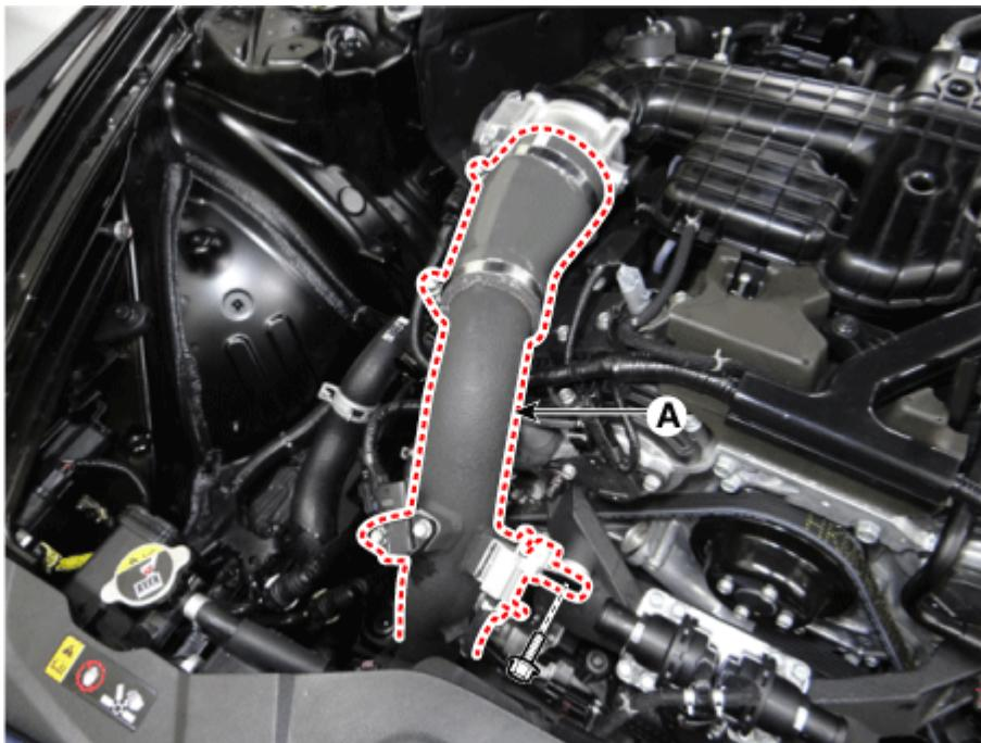
7. Remove the surge tank stay mounting bolt (A).
