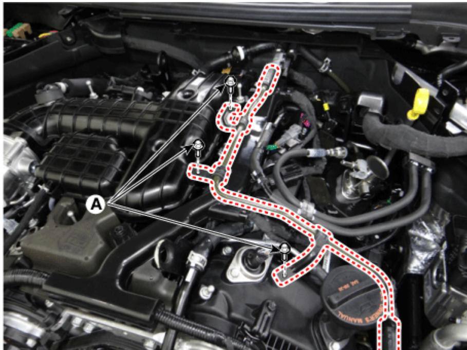
4. Disconnect the wiring connectors and harness clamps and remove the wiring protector around the surge tank.
