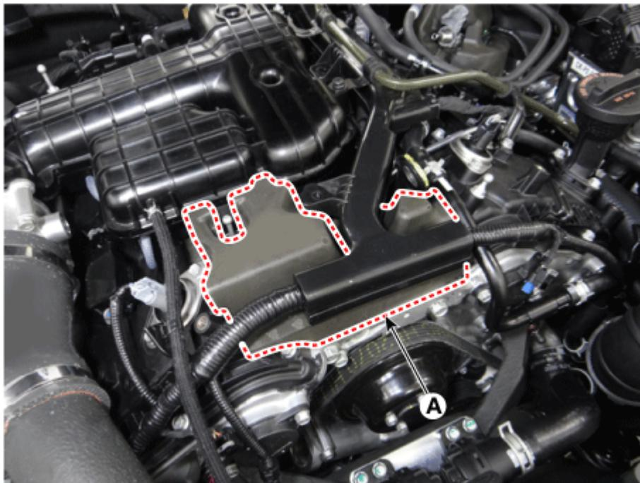
6. Disconnect the intercooler outlet hose.
