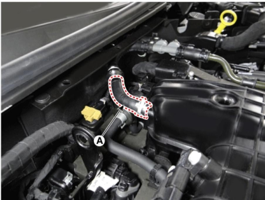
10. Separate the electric throttle control (ETC) module.
