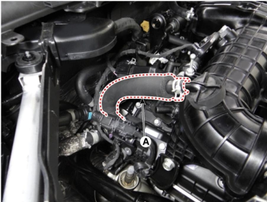
9. Disconnect the brake vacuum hose (A).
