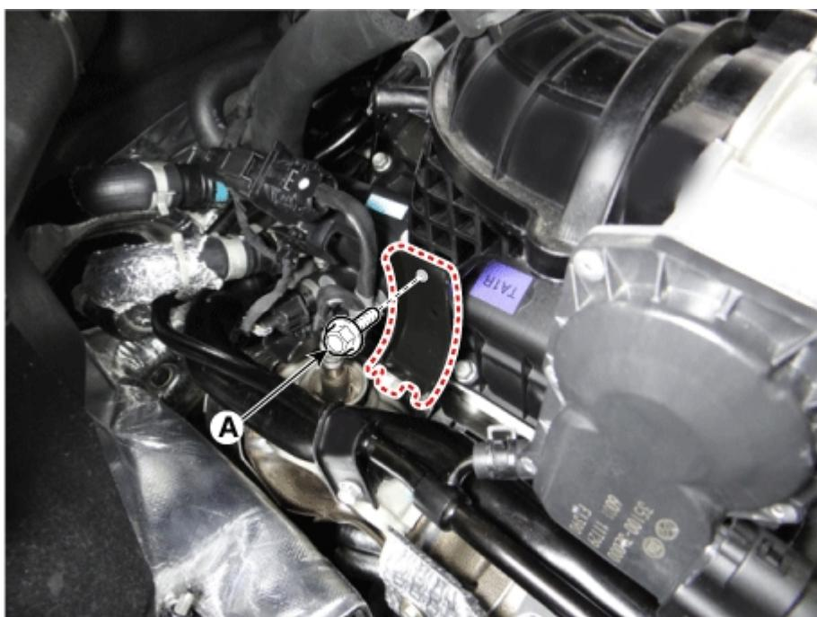
8. Disconnect the positive crankcase ventilation (PCV) hose (A).
